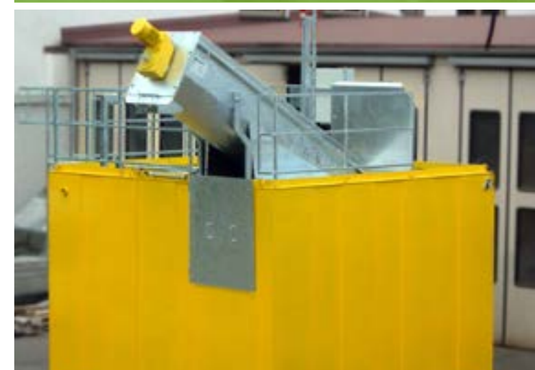
Version III: Mobile RWS in Stahlbecken integriert Mobile RWS integrated in steel tank
